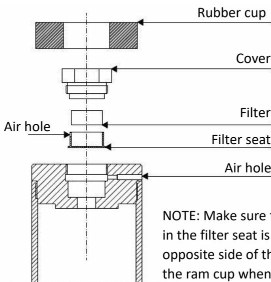
NOTE: Make sure that the hole in the filter seat is on the opposite side of the air hole in the ram cup when assembly.
